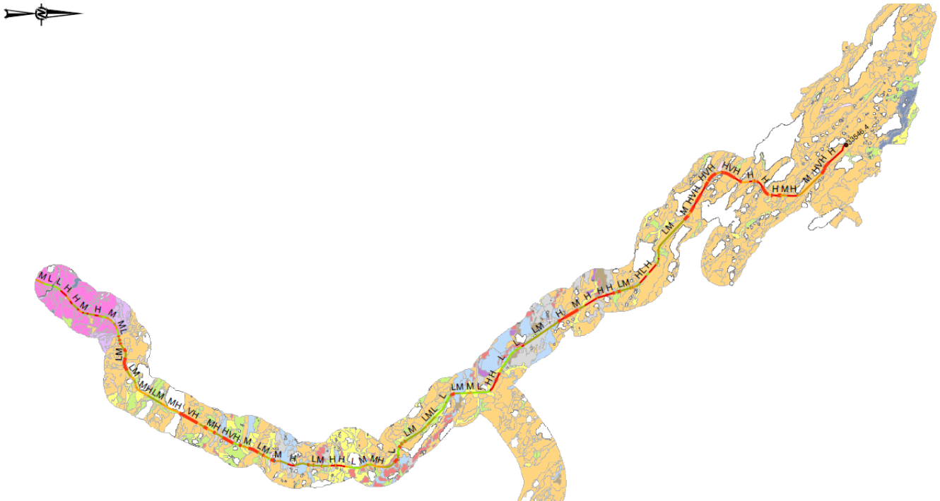
Figure 1: Risk of Thaw or Subsidence along Pipeline Route (Red is rated as High to Very High (H to VH) as discussed in text)
