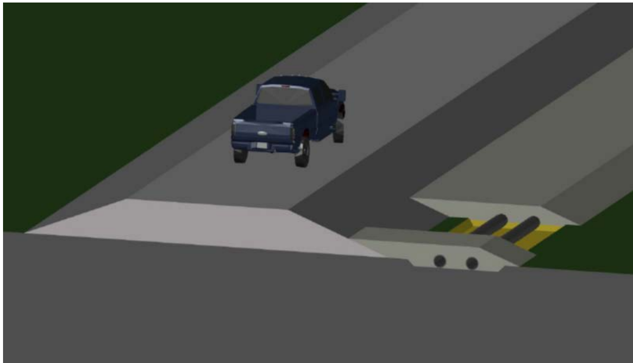
Figure BZ-TRC-01a. Conceptual design of waterline cover on the east side of the All Weather Access Road.
