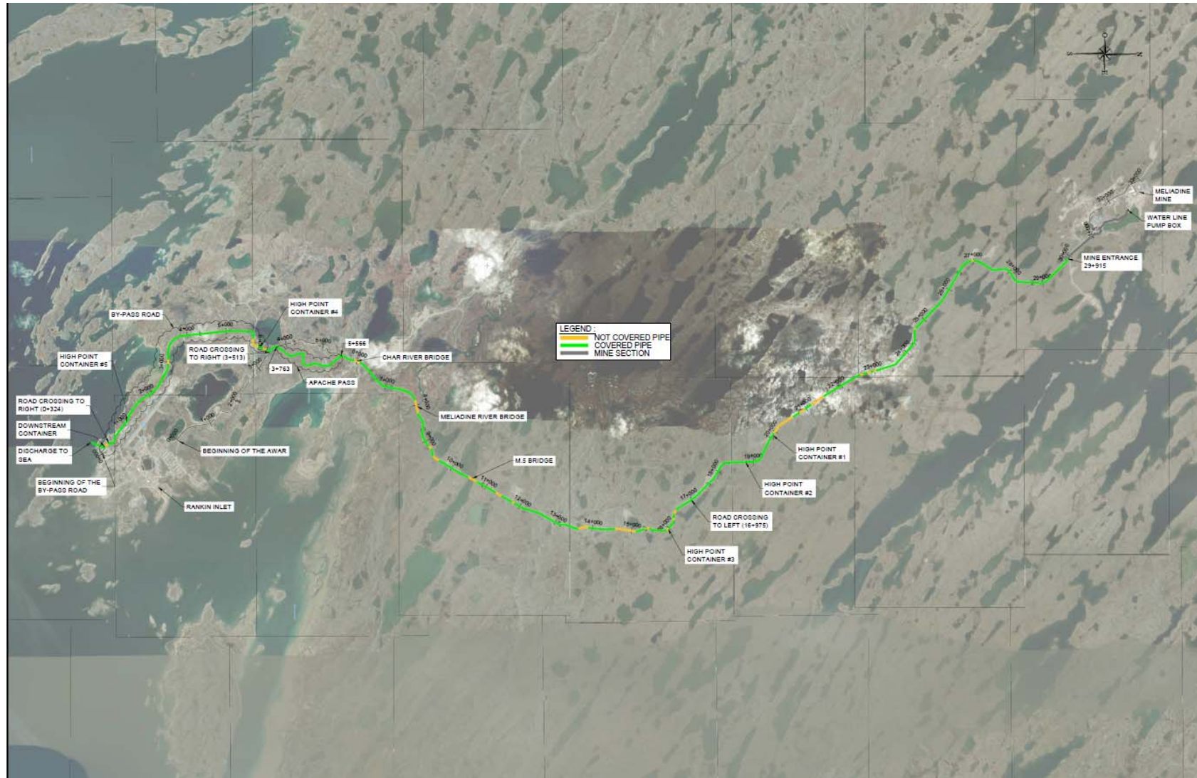
Figure 2: Waterline Layout (By-Pass Rd KP0+000 to KP6+000, AWAR KP3+763 to KP29+915, Mine KP29+915to KP32+000)
