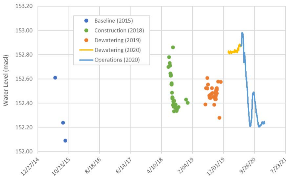
Figure 18 Measured water levels in Mammoth Lake. Results from 2015 – 2019 are by GPS survey, and results for 2020 are from piezometric data (3-h intervals).
