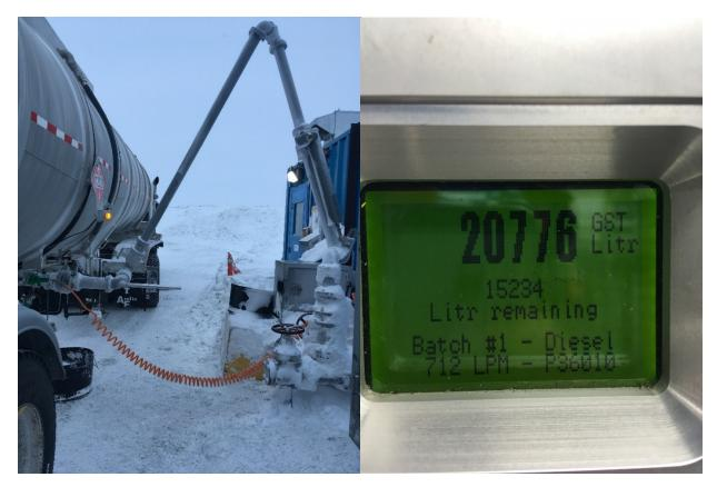
Photo 3: Agnico Eagle Ltd.'s Refueling Station – Loading arm and Scully System
