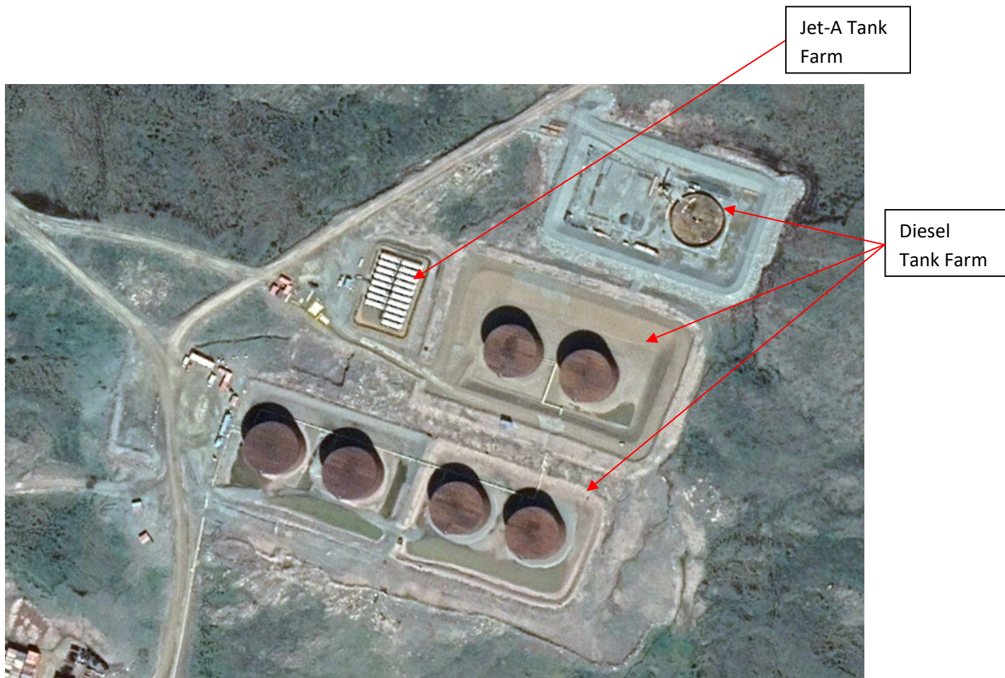
Figure 2 – Agnico's Baker Lake Bulk Fuel Storage Facility Site Layout
