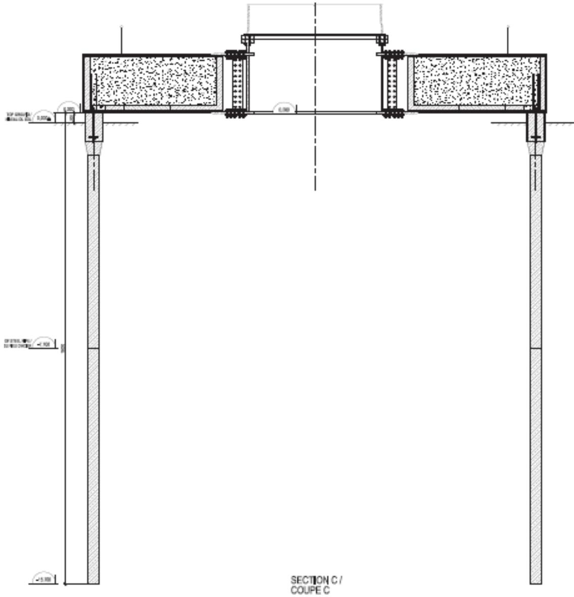
Drawings showing the concept of the steel spider foundation
