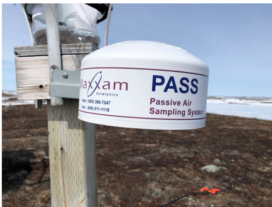
Figure 2-3. NO 2 -SO 2 sampler at the Meliadine site.
