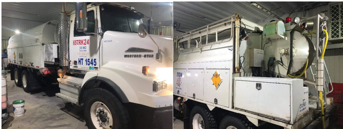
Figure 3-1 Mobile modular Emulsion Plant and Explosive Truck
