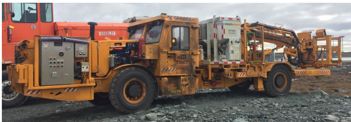
Figure 3-3 Underground Emulsion Charger – Dyno Loader
