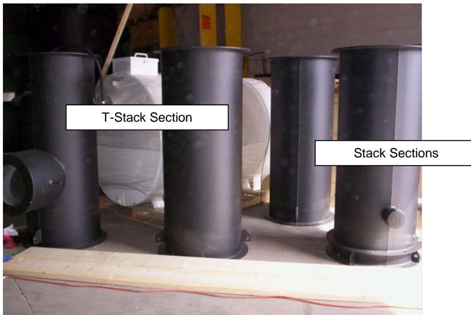
**T-Stack and Stack Sections**
