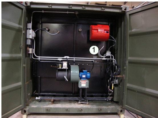
Primary Chamber Burner Flexible lines
