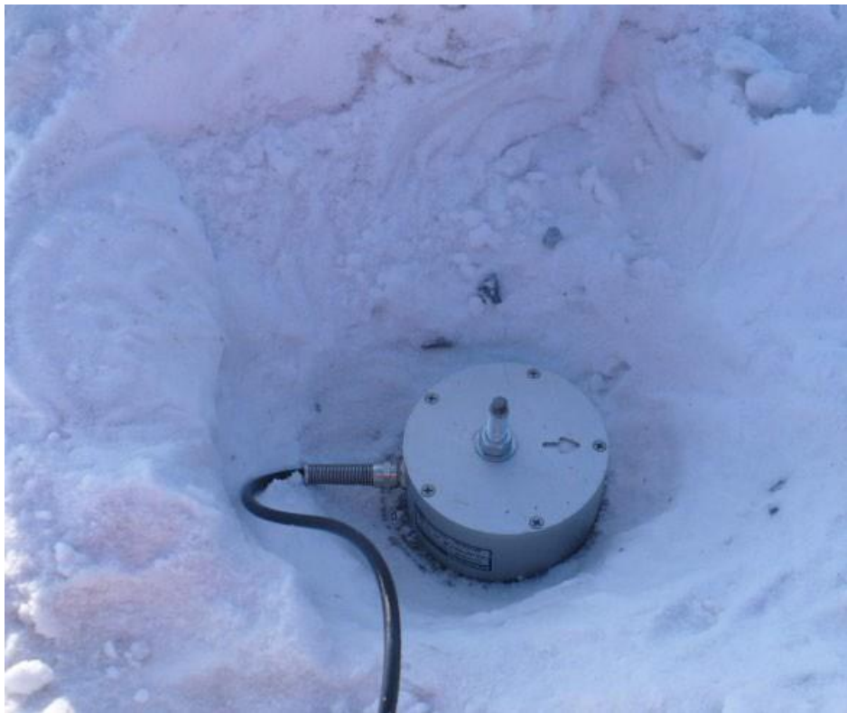
Figure 4 Transducer tightened with a nut
