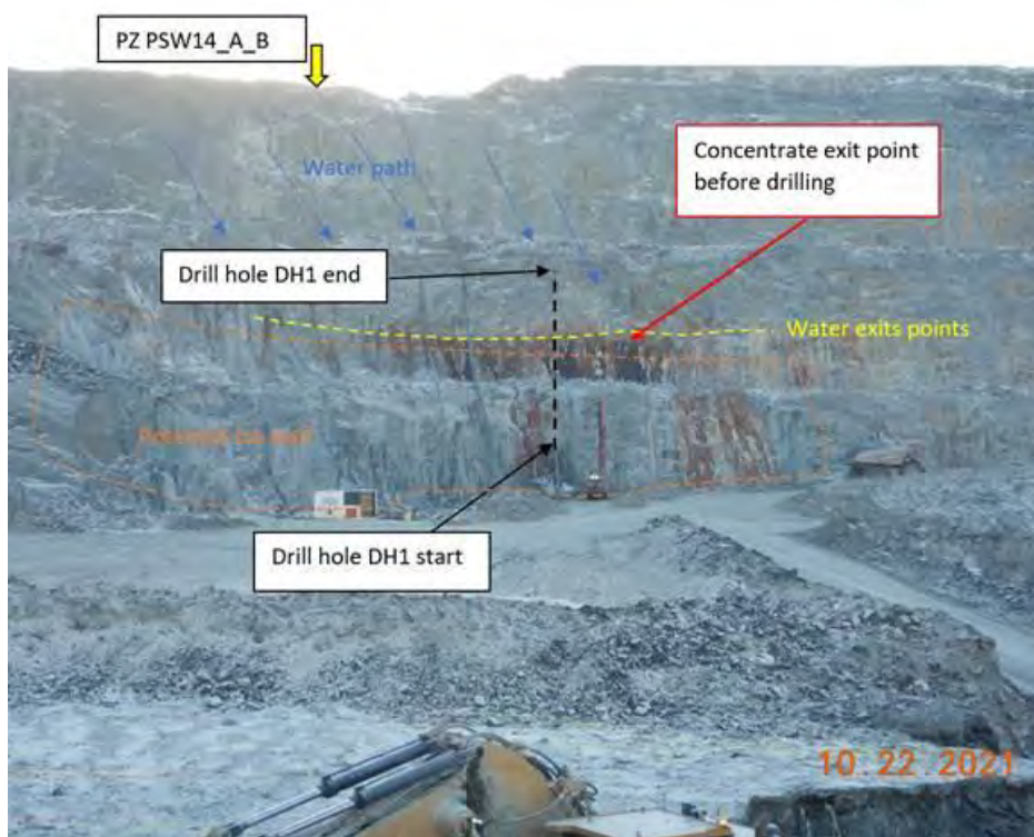
Photo 6: Pit seepage along south wall, looking south towards Drill hole-1 and seepage sample location ST-GW-WT-1 (October 22, 2021).
