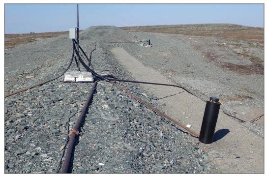
**Photo 5:** Dike D-CP1 - Crest—Center and downstream. GTC housing and datalogger.
