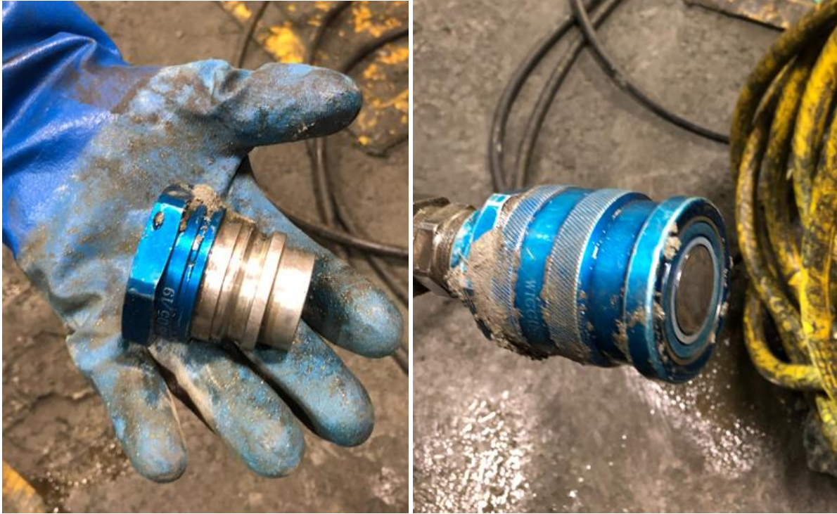
Figure 2: Broken hydraulic line connection from Fuel/Lubrication truck.
