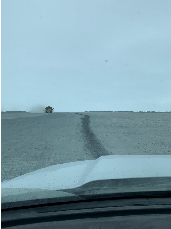
Figure 2: A hydraulic line ruptured on a haul truck and oil leaked between TIRI1 and WRSF1.
