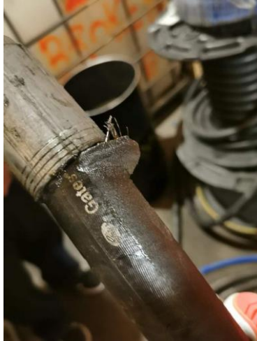
Figure 2: Failure of the hydraulic line of excavator.
