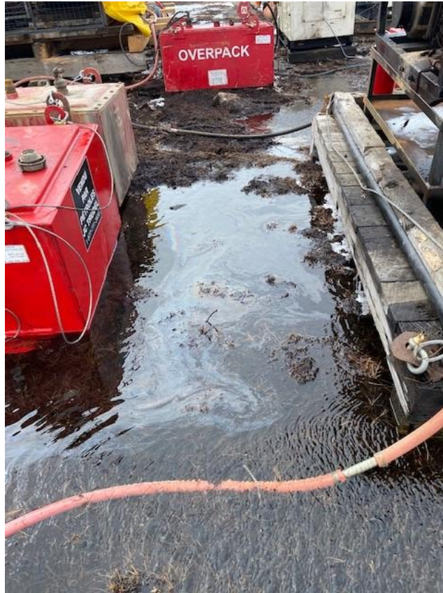
Figure 2: Hydrocarbons sheen on the surface of water by the drill
