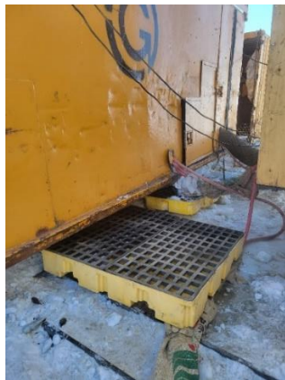
Figure 3: Spill tray installed under the drain hole
