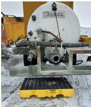
Figure 3: Secondary containment is now available with the drill cutting vacuum pump
