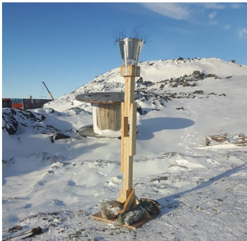
Figure 2. Dustfall sampling stand at the Meliadine site.
