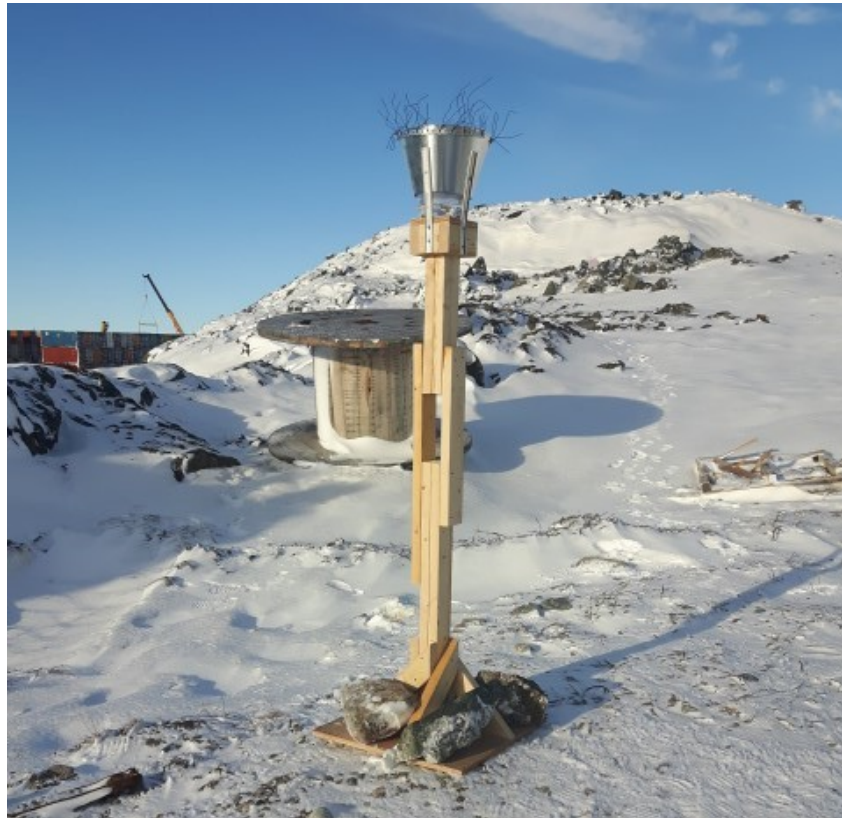
Figure 2. Dustfall sampling stand at the Meliadine site.
