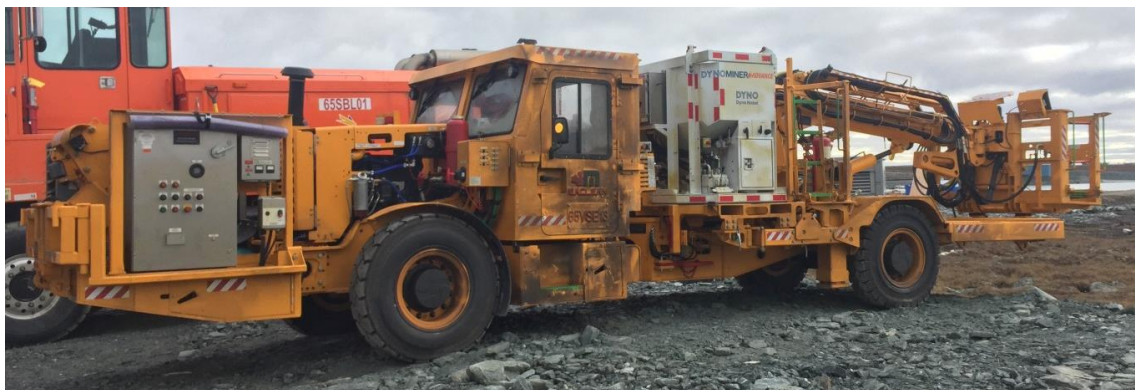
Figure 3-3 Underground Emulsion Charger – Dyno Loader
