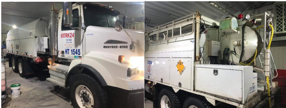
Figure 3-1 Mobile modular Emulsion Plant and Explosive Truck
