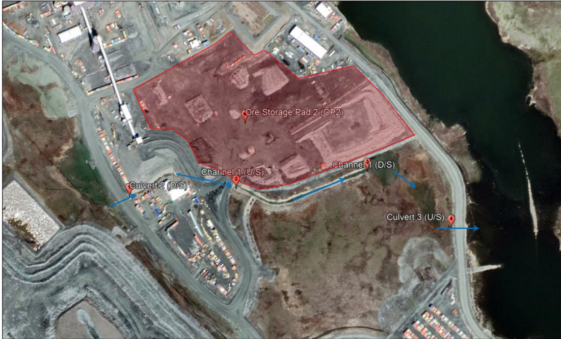
Figure 9: Locations of EC monitoring stations relative to OP2 (red polygon) and the general flow path from Culvert 2 to Culvert 3, and ultimately CP1 (blue line).
