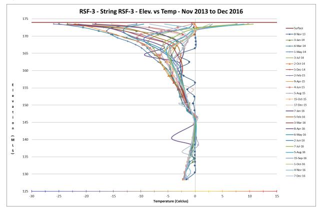
Figure 31. Thermistor Results RSF-3
