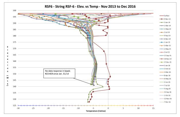
Figure 34. Thermistor Results RSF-6
