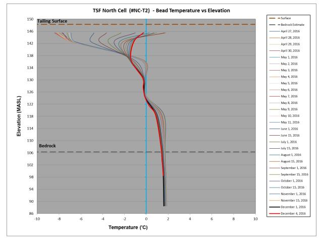
Figure 22. Thermistor Results NC-T2
