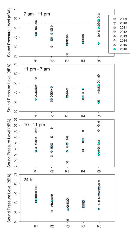
Figure 43.  $L_{eq}$  values calculated from filtered data for various time periods at locations R1 – R5 on the Meadowbank site in surveys from 2009 - 2016. Dashed lines indicate target sound levels (day-time and night-time only).
