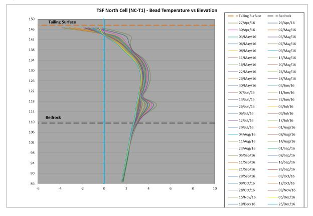
Figure 21. Thermistor Results NC-T1
