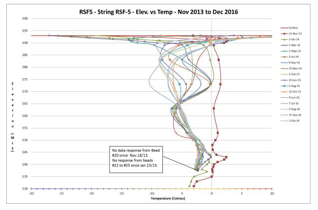
Figure 33. Thermistor Results RSF-5
