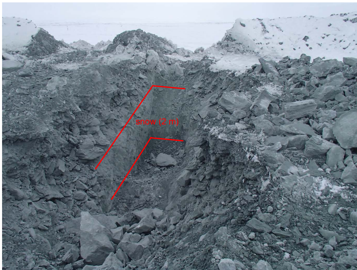
Photograph NCIS-001: View of a test pit in the UM rockfill lift at El. 152 m: a thick layer (2 m) of snow underlies the rockfill.
