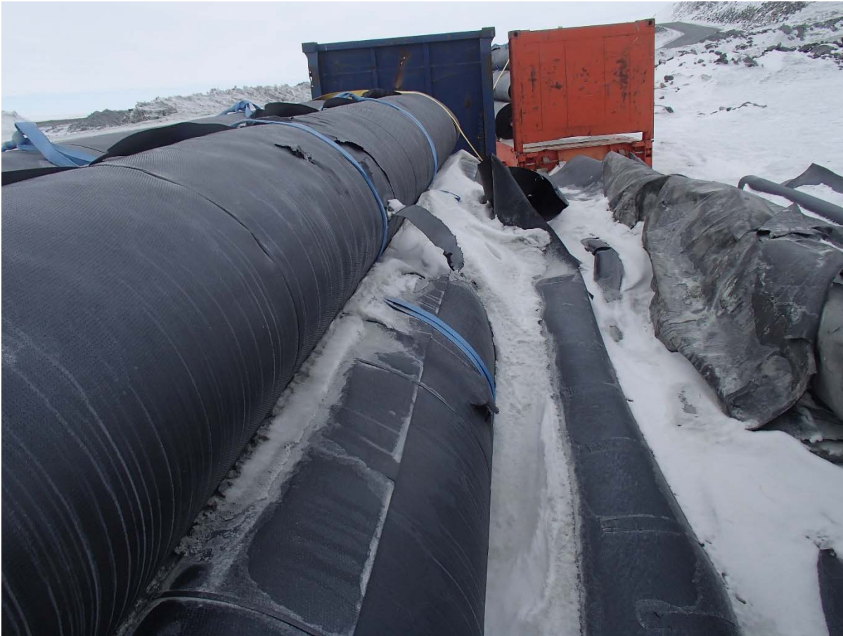
Photograph from the LLDPE storage site: View of new rolls stored on a trailer, showing tears.
