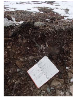
NCIS-015 (2018-05-22), looking S from Sta. 1+850 m. View of the 200 mm deep test pit excavated into the natural soil. A thin layer or organic soil overlies frozen till.
