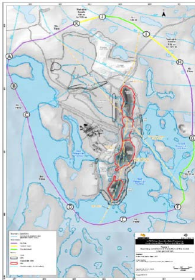
Figure 3-4: Flow Boundary Conditions (at the bottom of the model, sub permafrost conditions)
