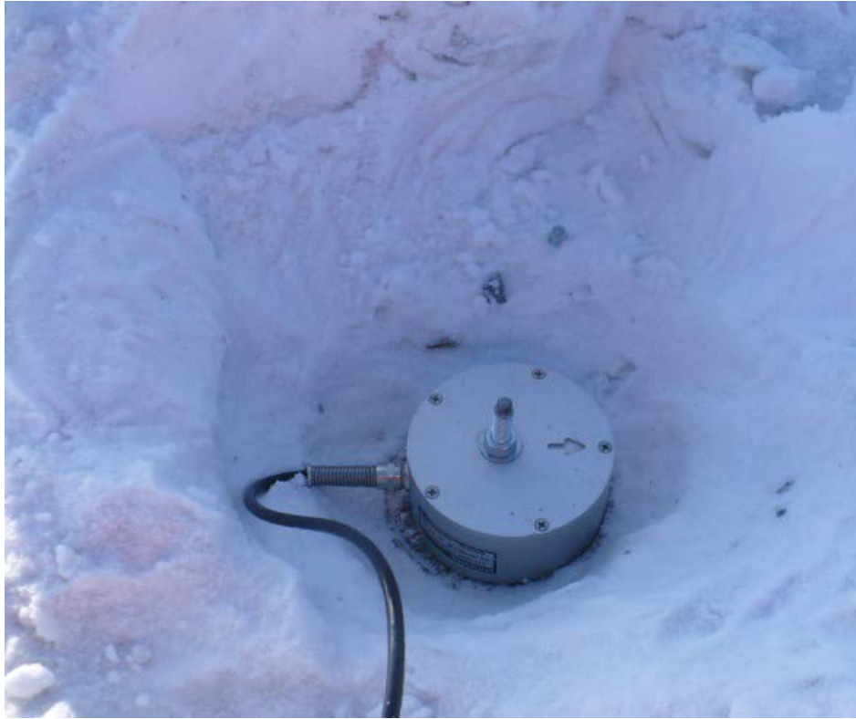
Figure 4: Transducer tightened with a nut
