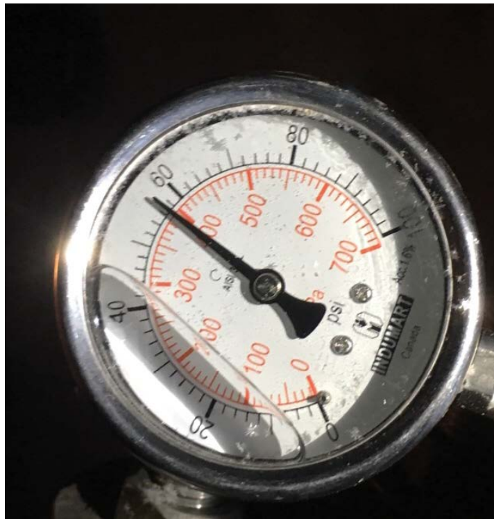
Picture 10 Pipeline pressurization
