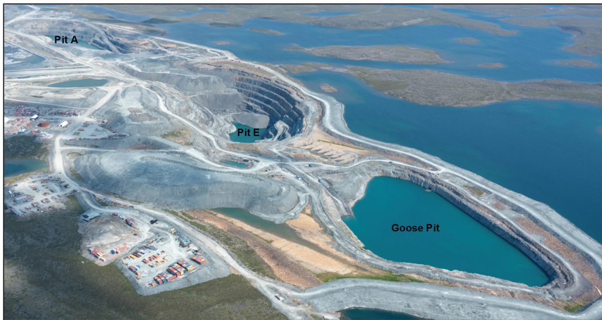
Figure 3-18: In-Pit Area for Tailings Management (Summer 2020)
