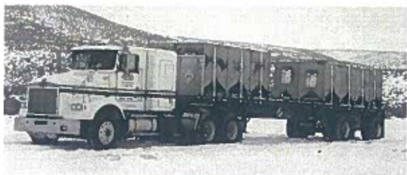
Figure 11. Bins corded two abreast on a flatbed trailer. The bins are strapped to the trailer to prevent movement during transportation.
