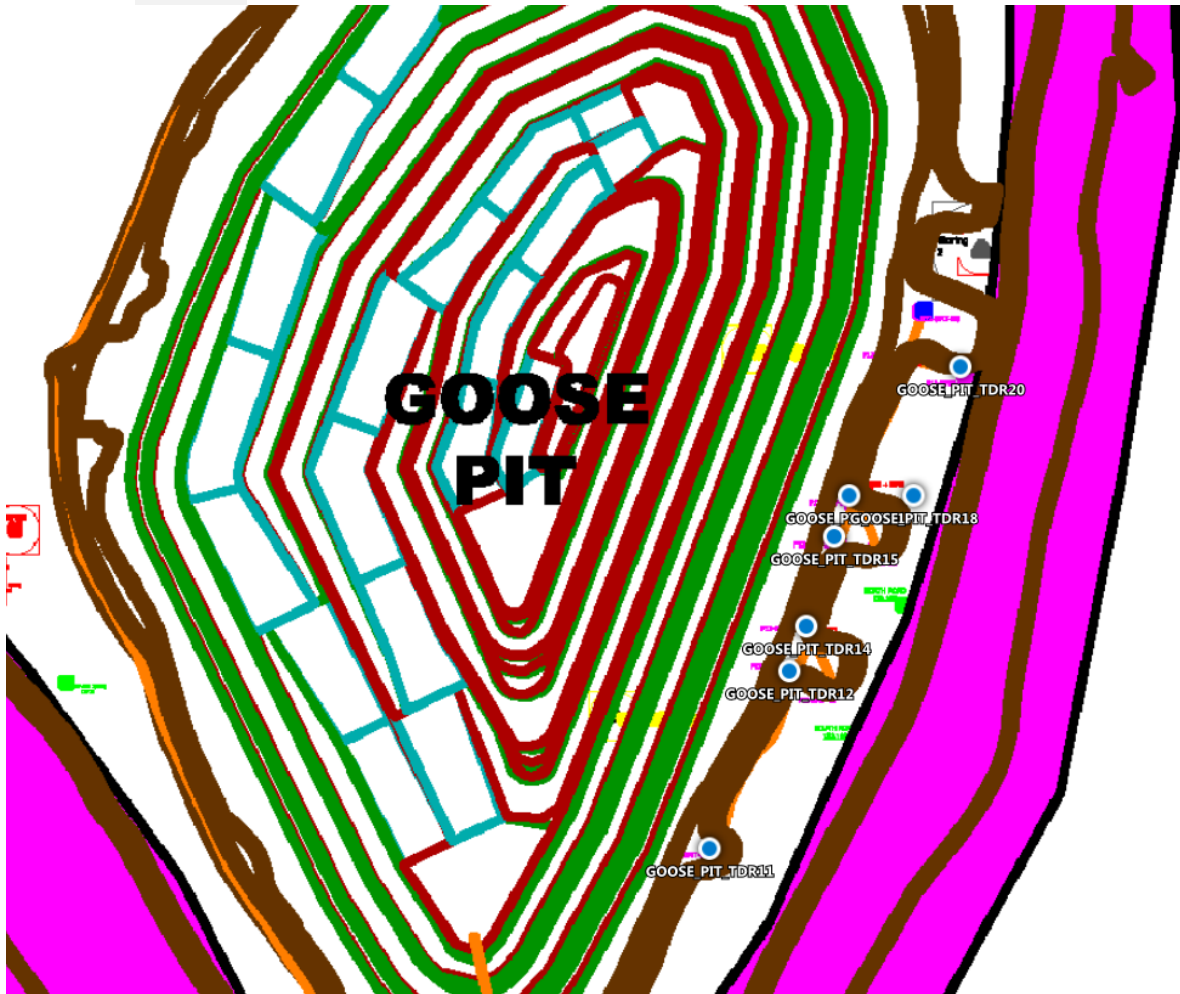
Figure 6: Location of downhole instruments at Goose pit
