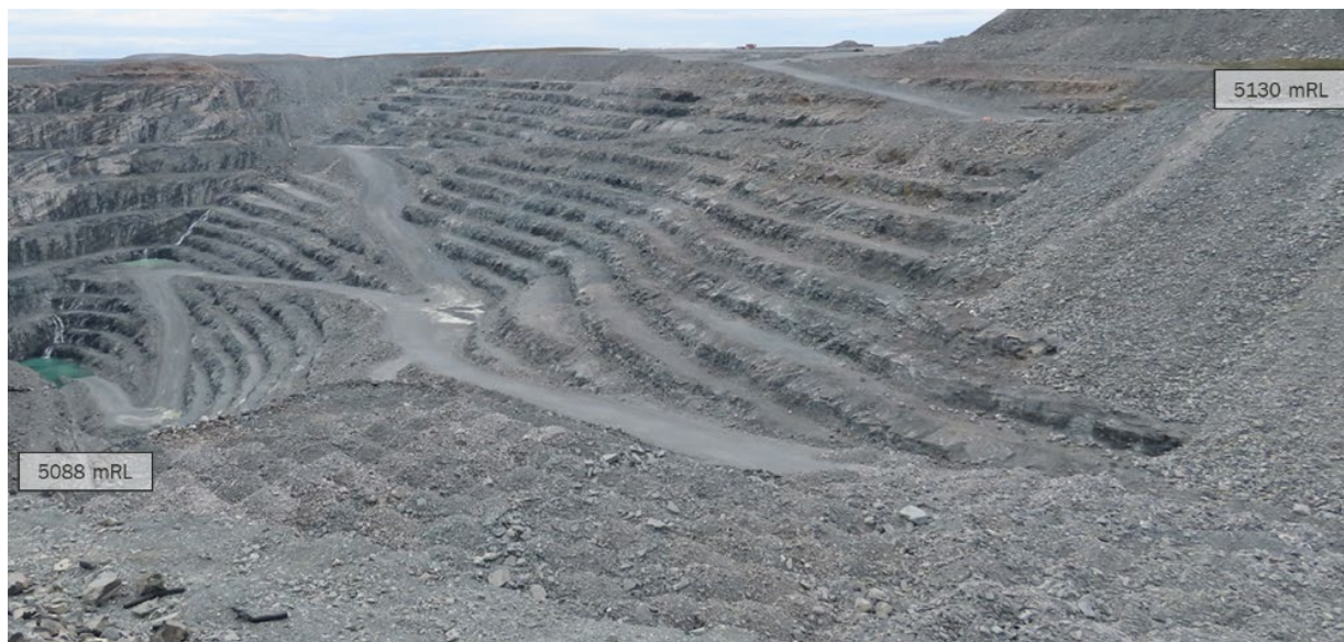
Photograph 8-6: Vault Pit west wall looking south (2019) showing dump advance
