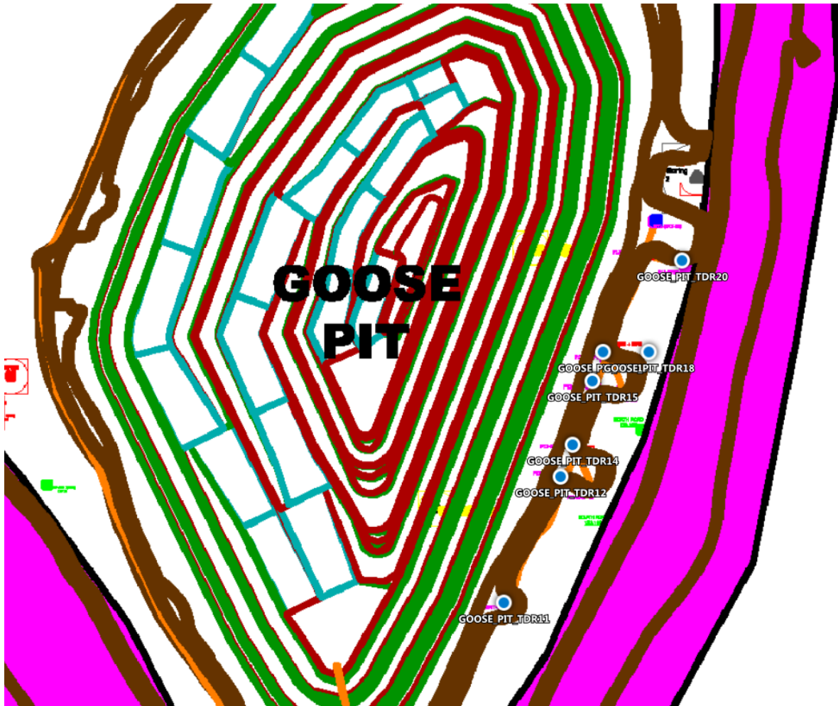
Figure 67: Location of downhole instruments at Goose pit
