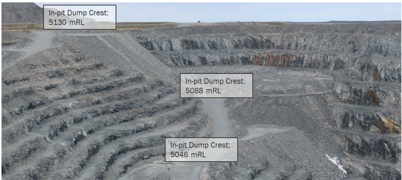
Photograph 8-15: Vault In-Pit dumps
