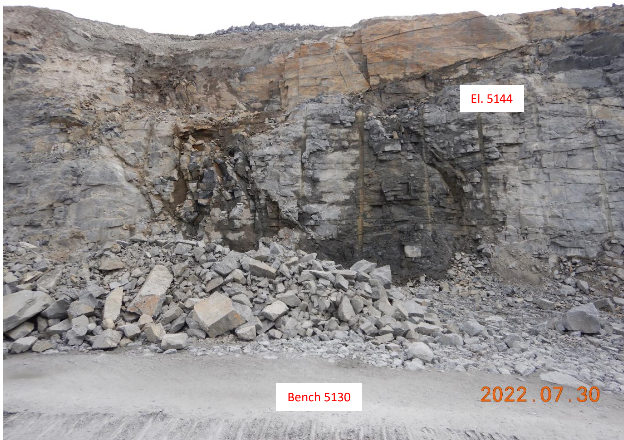
Photo 2: Pit seepage along Whale Tail Pit south wall, concentrated water source type, flow observed from the top layer and joint set / fault brittle structure (water source is related to ongoing water management operations), looking south (July 30, 2022).
