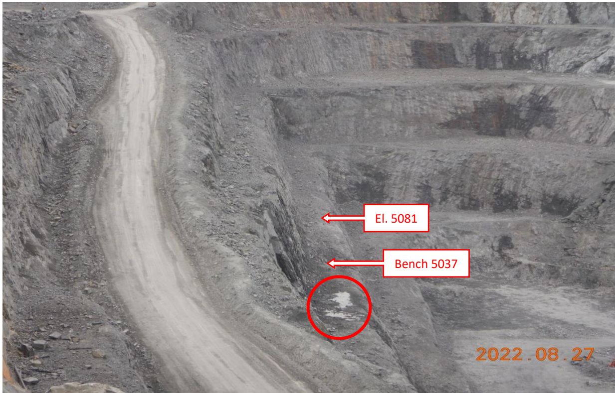
Photo 4: Whale Tail Pit, looking southwest, water accumulation on the catchment later in August 2022; this picture was taken without fresh rain (August 27, 2022).
