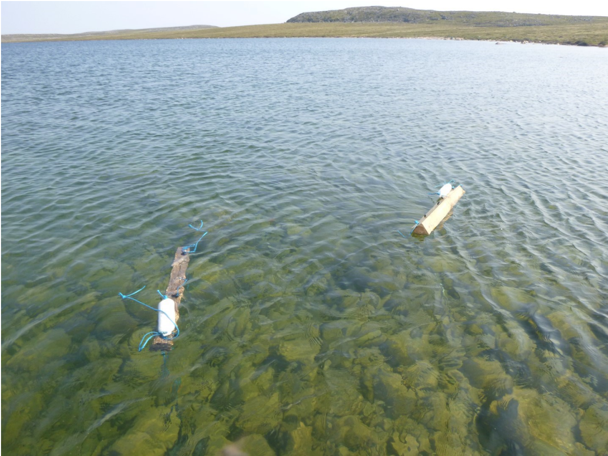
Figure 4. Artificial substrate periphyton sampler in-situ.
