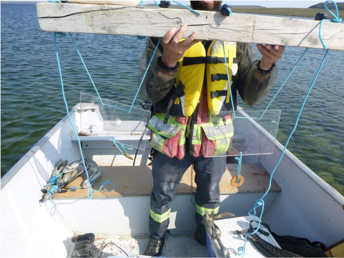
Figure 3. Artificial substrate sampler for periphyton pilot study in 2022.
