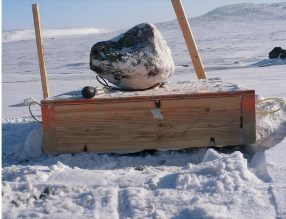
Figure 5: Final Set-up with the Microphone in the direction of the blast
