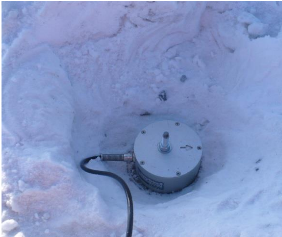
Figure 4: Transducer tightened with a nut
