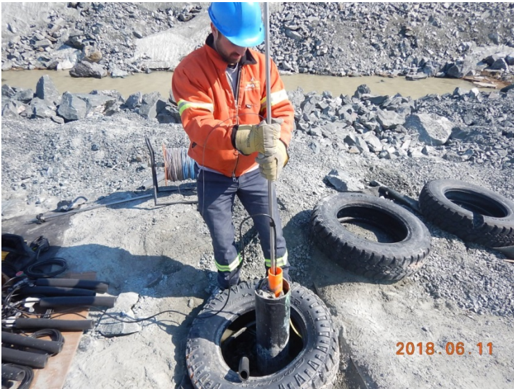
Photo 3.6: Connecting tube gently slid down the casing.
