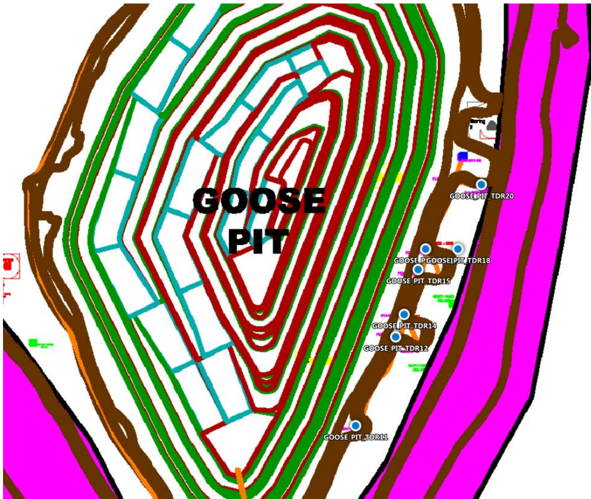
Figure 7: Location of downhole instruments at Goose pit
