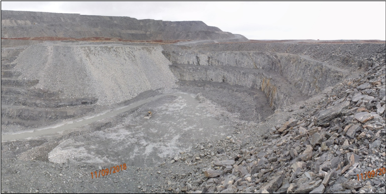
Photograph 8-12: Northeast through north transition wall (2018) and dump platforms at 5088 mRL and 5130 mRL
