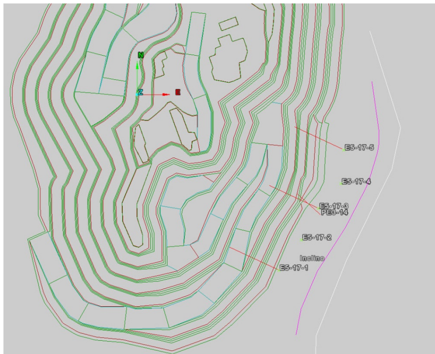
Figure 3: Location of Pit E instrumented holes collars
