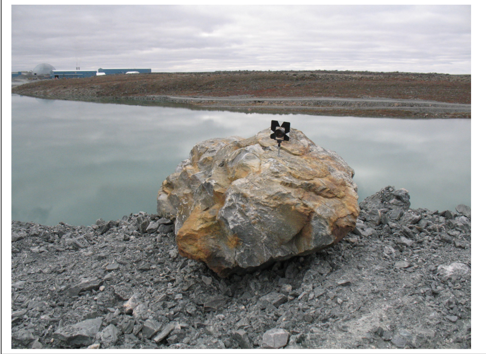
Photo #3 Typical survey prism mounted on large boulder
