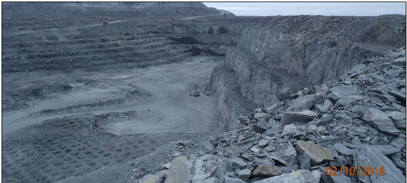
Photograph 8-8: Typical bench crests along highwall
