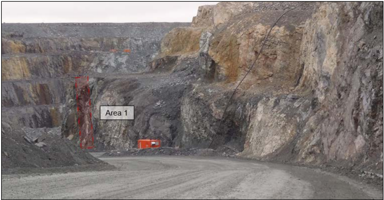
Photograph 6-8: Pit E3 Ramp Area 1 above ramp - Bay Fault or splay (2016)
