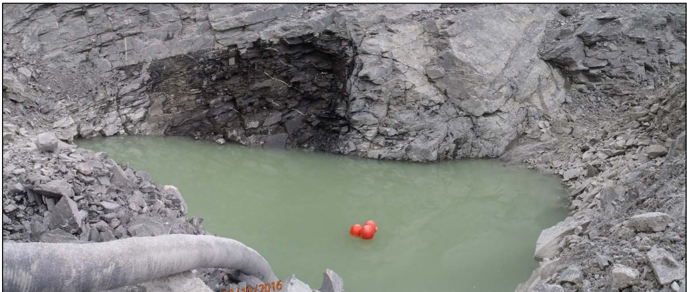
Photograph 8-6: Sump at southwest corner of Vault pit
