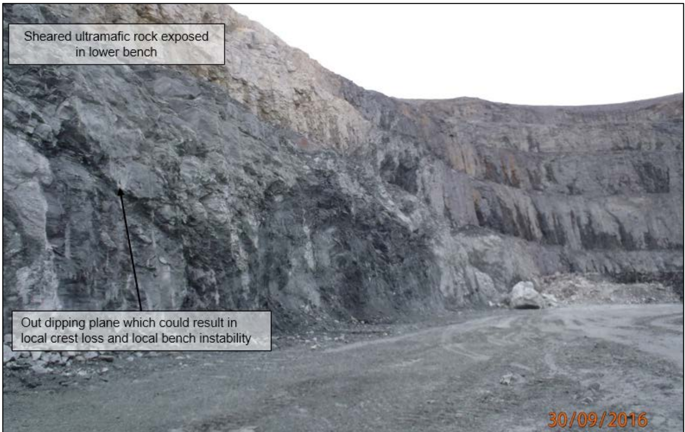
Photograph 4-6: Ultramafic rock exposed at toe of Pit A west wall
