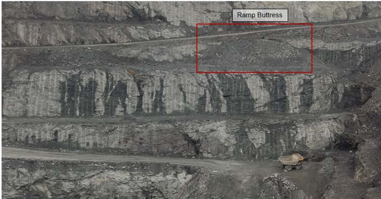
Photograph 6-15: Pit E3 west wall ramp buttress and step-in (2016)
