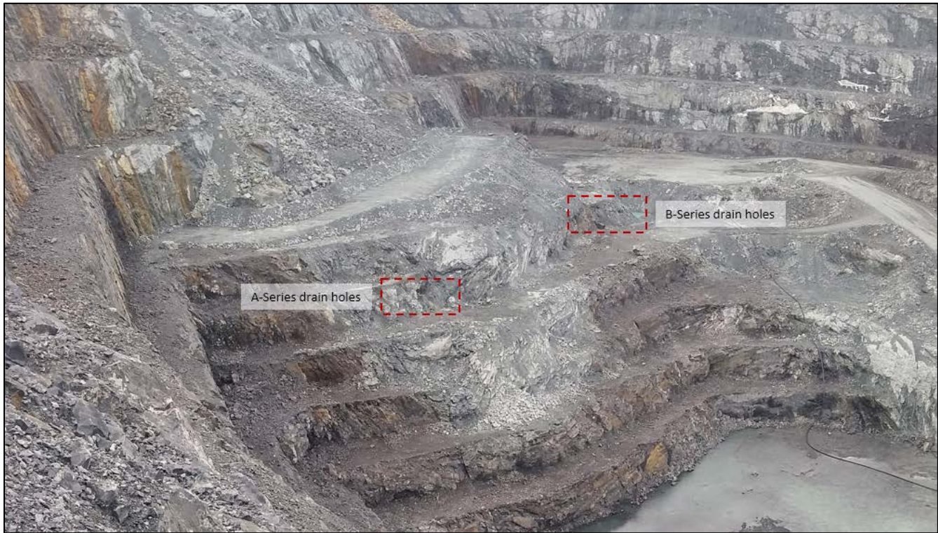
Photograph 6-4: Approximate location of the A-series and B-series of drain holes (2016)
