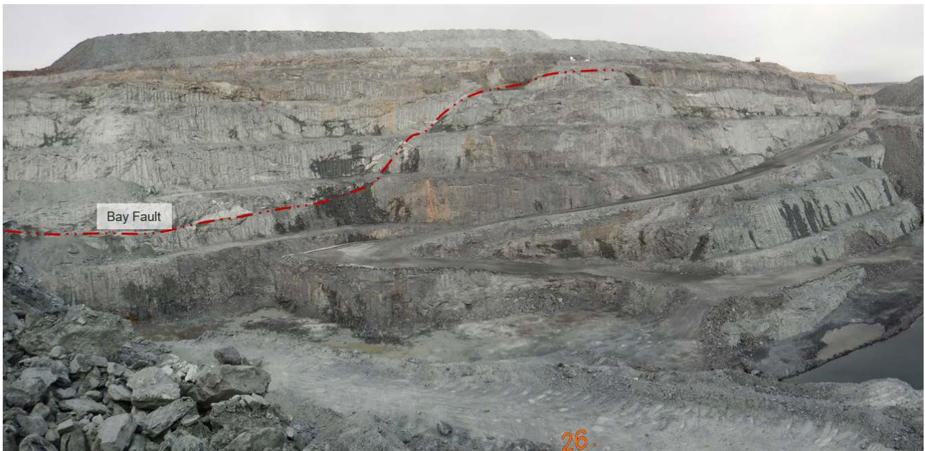
Photograph 6-11: Pit E west wall showing seepage and Bay Fault (2017)
