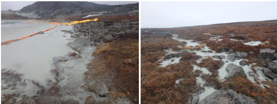
Photo 1: NP1 Lake Visual observation of the TSS exceedance, taken on June 6 th .
