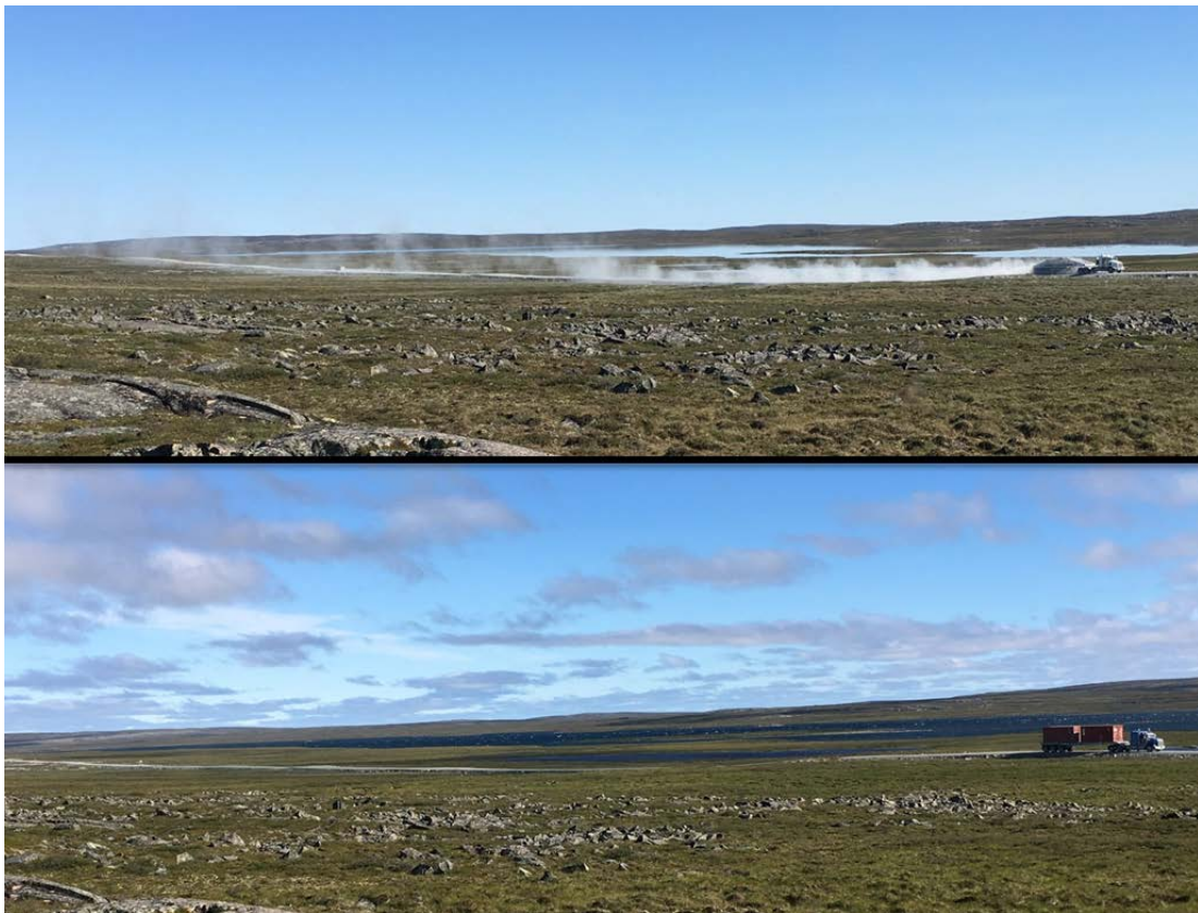
Figure 2. Dust generation in the TETRA Flake test area (km 10 – 12) before (top) and after (bottom) application.
