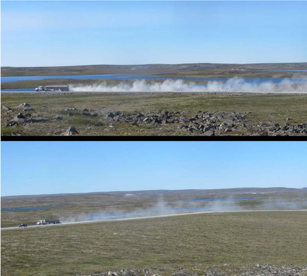
Figure 4. Dust generation in the speed limit test area (km 24-26) at 50 km/h (top) and 40 km/h (bottom).
