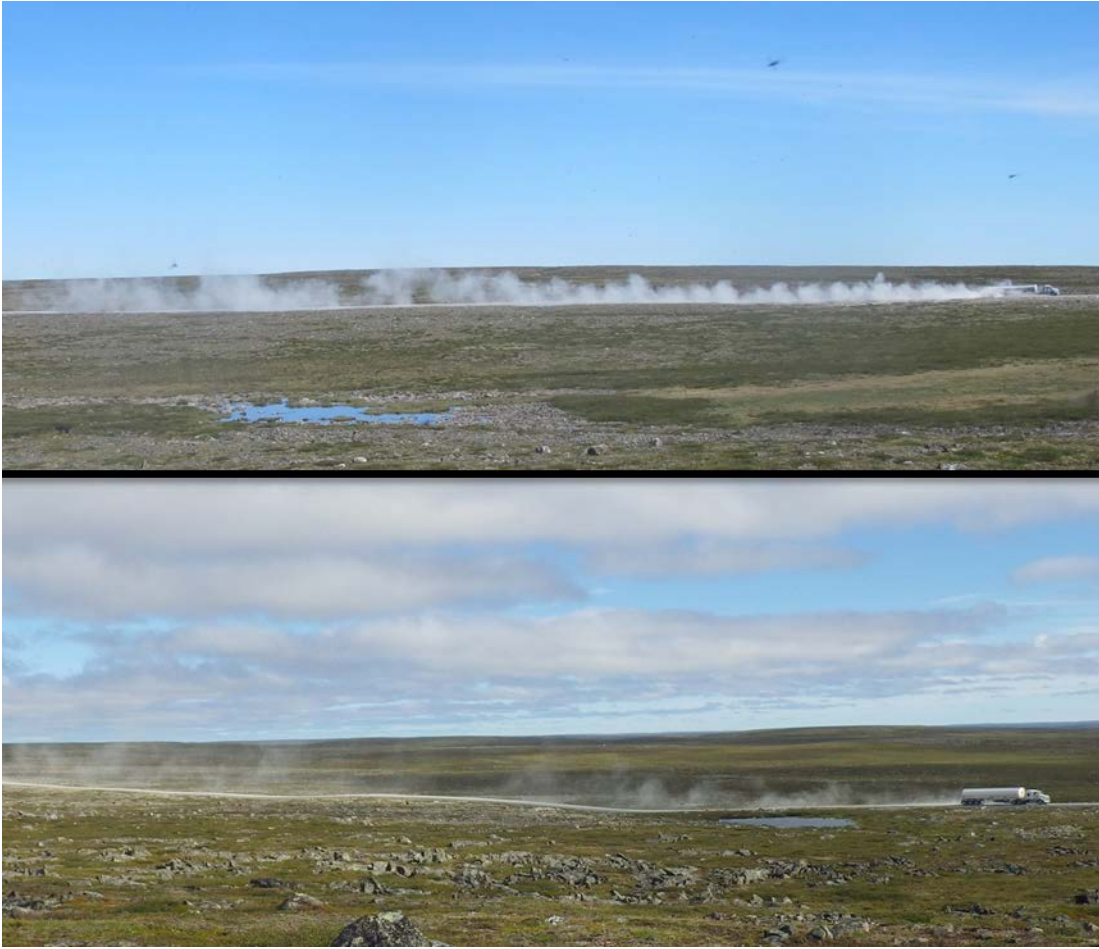
Figure 3. Dust generation in the Dust Stop™ test area (km 48 – 50) before (top) and after (bottom) application.
