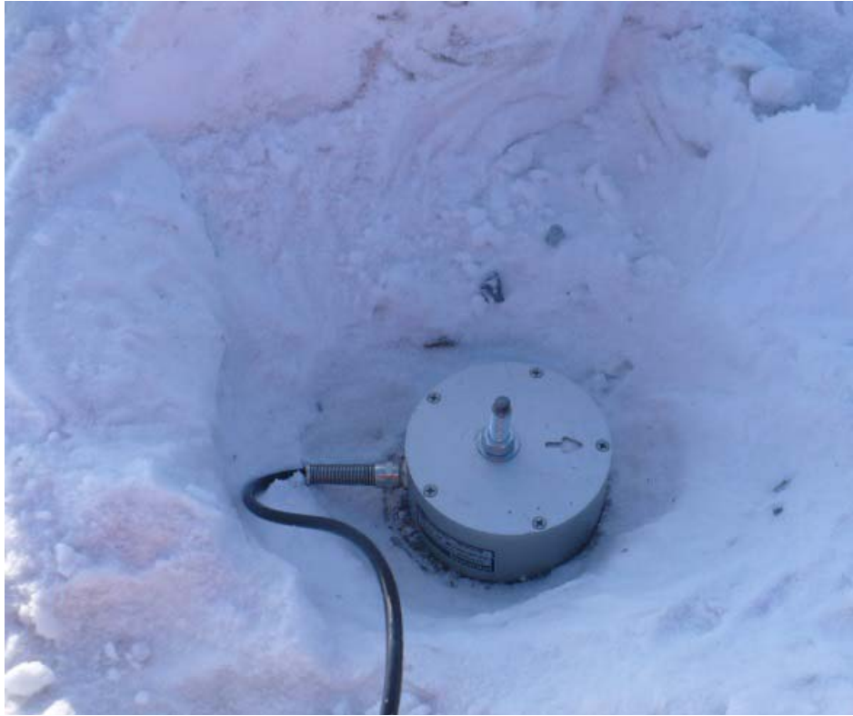
Figure 4: Transducer tightened with a nut
