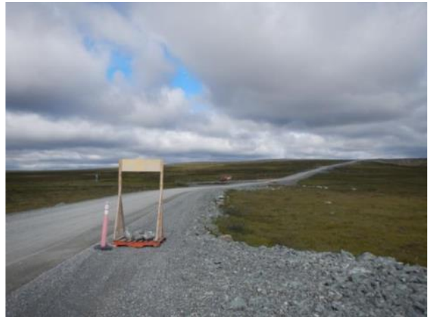
Photo 46: Dust test study area number three located near km 48: use of Dust Stop
