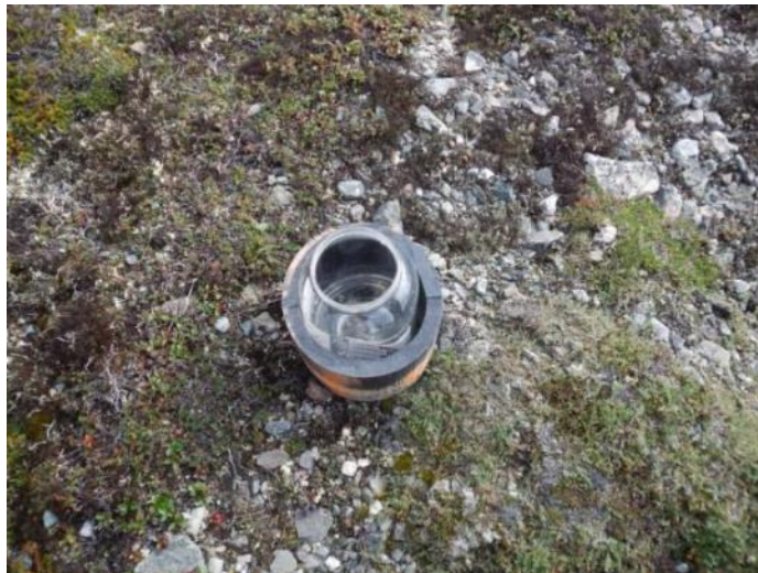
Photo 44: Dust Sampling Station
