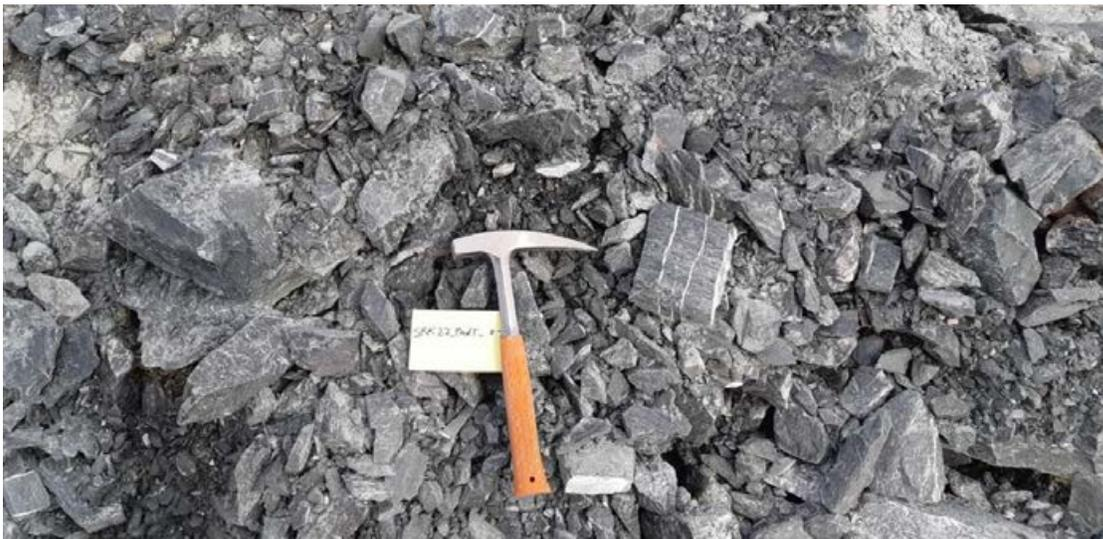
Figure 5-2: SRK22-PadT-07; showing dark gray mafic metavolcanics (1a) with carbonate veining
