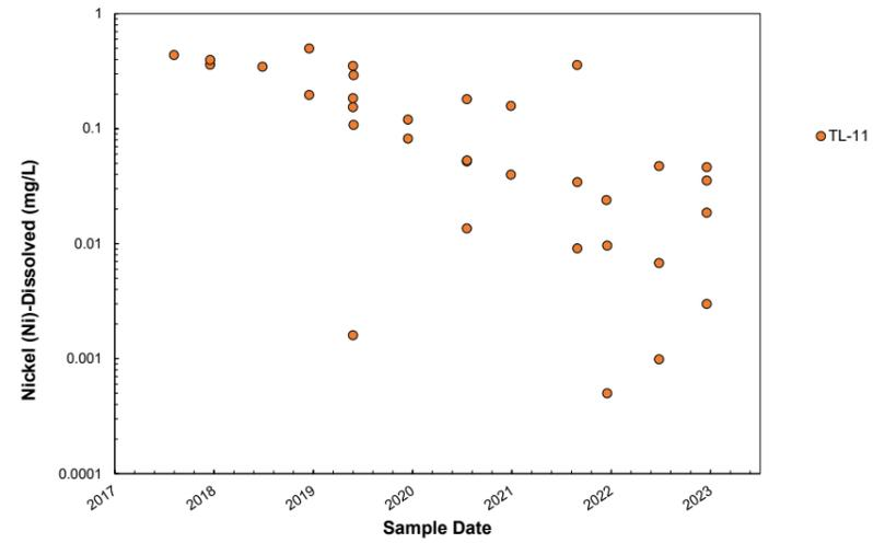
Figure 8-7: Nickel timeseries plot for underground seepage (TL-11)
