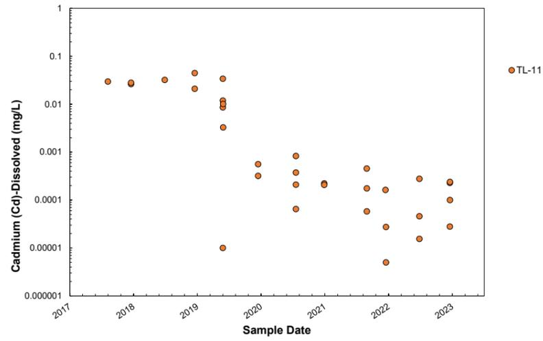
Figure 8-4: Cadmium timeseries plot for underground seepage (TL-11)
