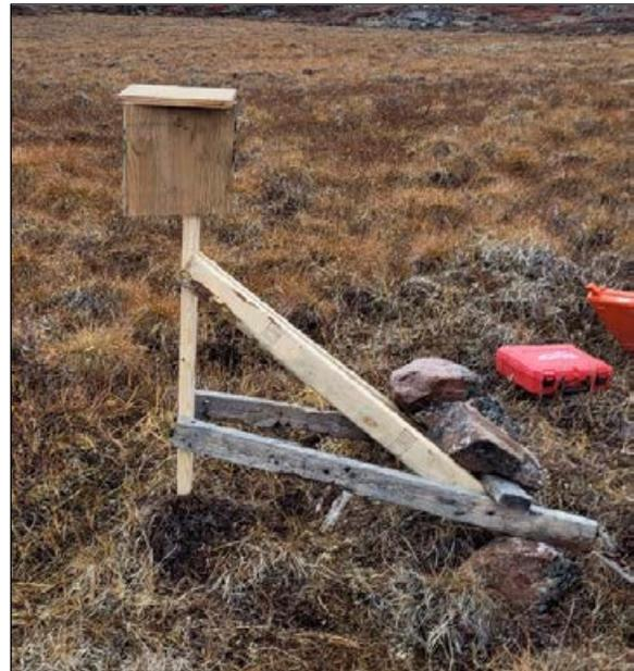
**Photo 3.3-1: Doris camera 3 tripod repair. September 22, 2022.**
