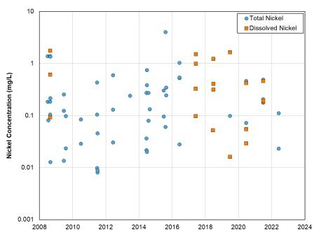
Figure 4.6: Seepage nickel concentrations
