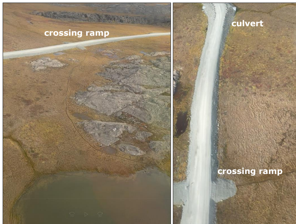
Photo 6 Aerial view of caribou crossing ramp with trails (left), and culvert where two additional cameras were deployed to monitor caribou activity in relation to crossing ramp (right) on Windy Road, August 2022.
