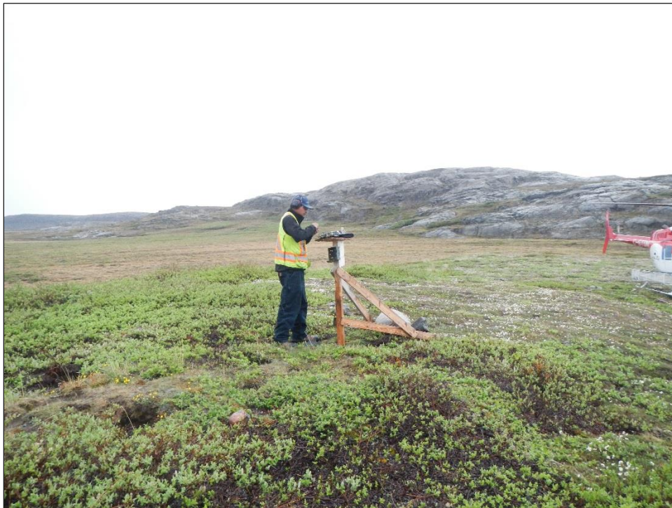
Photo 3.2-1 Example of camera set up camera height approximately 1.2 m).
