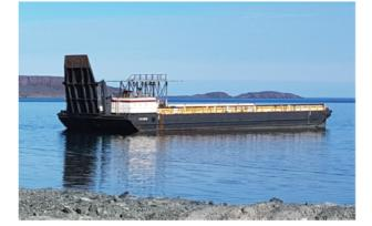
The FM 503 is a versatile ramp equipped deck barge. The barge was completely refurbished in 1998 adding a helicopter landing pad and new hydraulic bow ramp. The 503 has been utilized as a helicopter support barge, cable-laying vessel, and coastal equipment barge. She has generators and hydraulics on board as well as two large capacity pumps for the ballast system. The 503 is equipped as an oil spill response barge and has capacity to store 1500 M3 of recovered oil.
