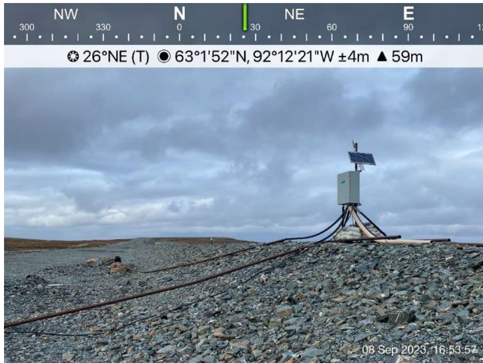
D-CP1 - Photo 5: Dike D-CP1: Ground temperature cable housing and data collection system.
