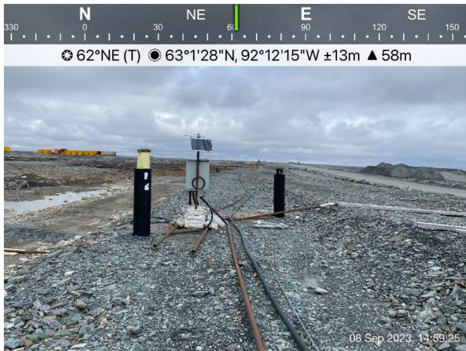
CP5 - Photo 4: Dike D-CP5 - Looking northeast, GTC housing and data collection system.
