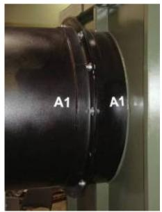
**Correctly Installed Breech on Primary Chamber**
