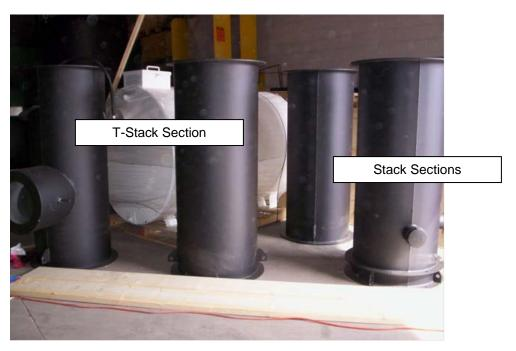
**T-Stack and Stack Sections**
