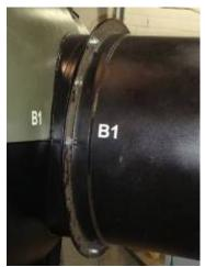
**Correctly installed Breech on Secondary Chamber**
