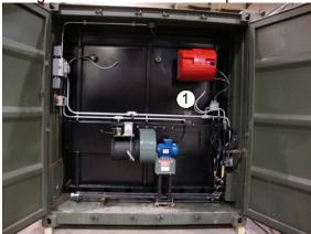
**Primary Chamber Burner Flexible lines**
