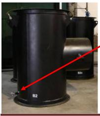
3. Stack Thermocouple on Stack
