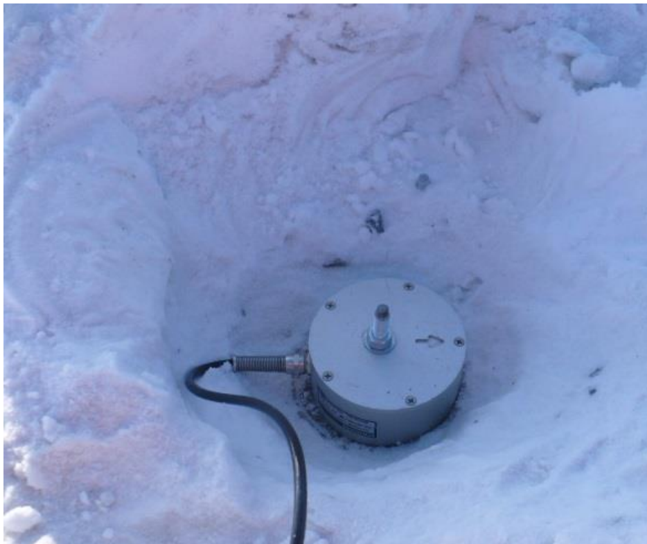
Figure 4: Transducer tightened with a nut
