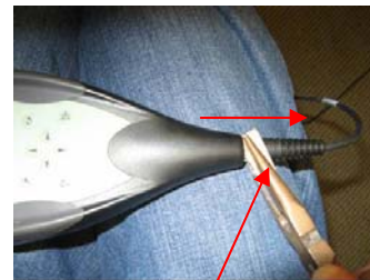
Use pliers to gently pull back sleeve.
