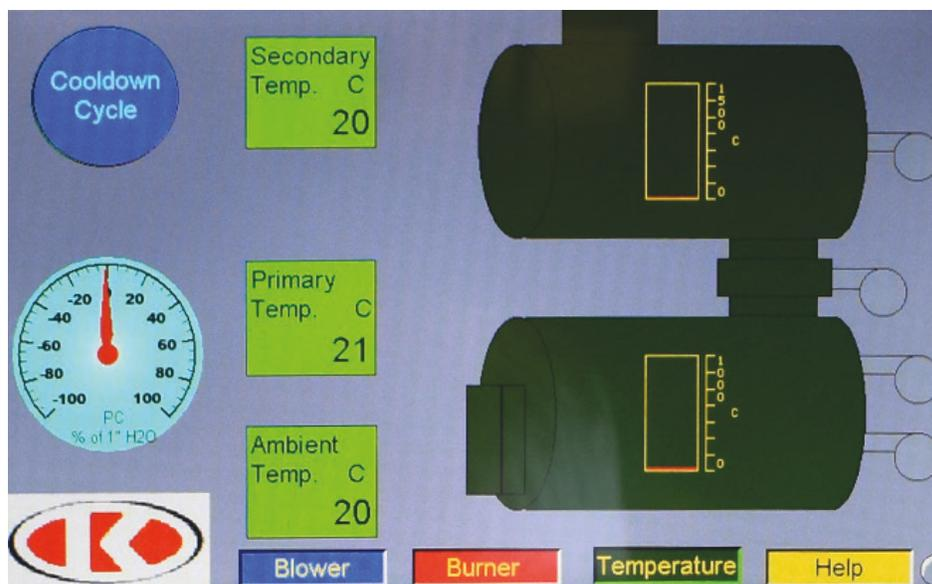
18. After secondary burners shut down, all the blowers will keep running for another 5-6 hours to give enough time for the incinerator to cool down and prevent any damage to the burners. If after the cool down process the temperature in the chambers is still above 250°C, the blowers will continue to run until the temperature drops below the 250°C value.
