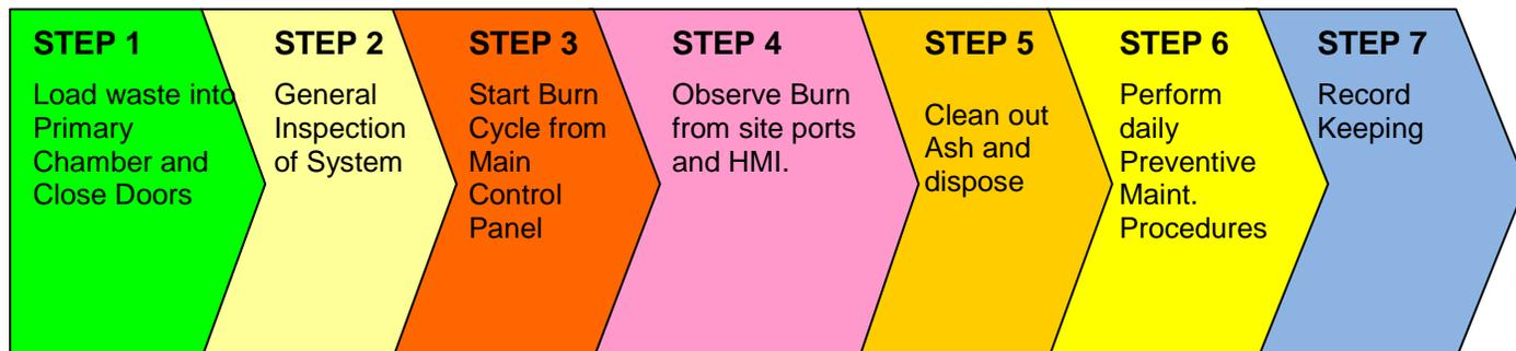
Although all 7 steps are critical in the general operation of the incinerator system, this section of the manual focuses on **Step 1**, **Step 3** and **Step 4** and how to start the system and monitor it during operation.
