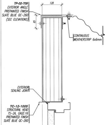
107.1 **HEADER ASSEMBLY ON NON-INSULATED WALL FOR STEEL DOOR** SCALE 1:5
