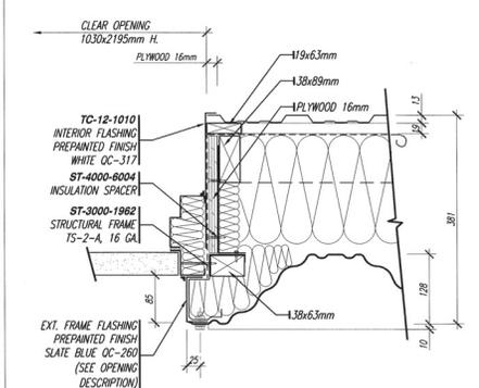
107.5 **VERTICAL ASSEMBLY FOR STEEL DOOR** SCALE 1:5
