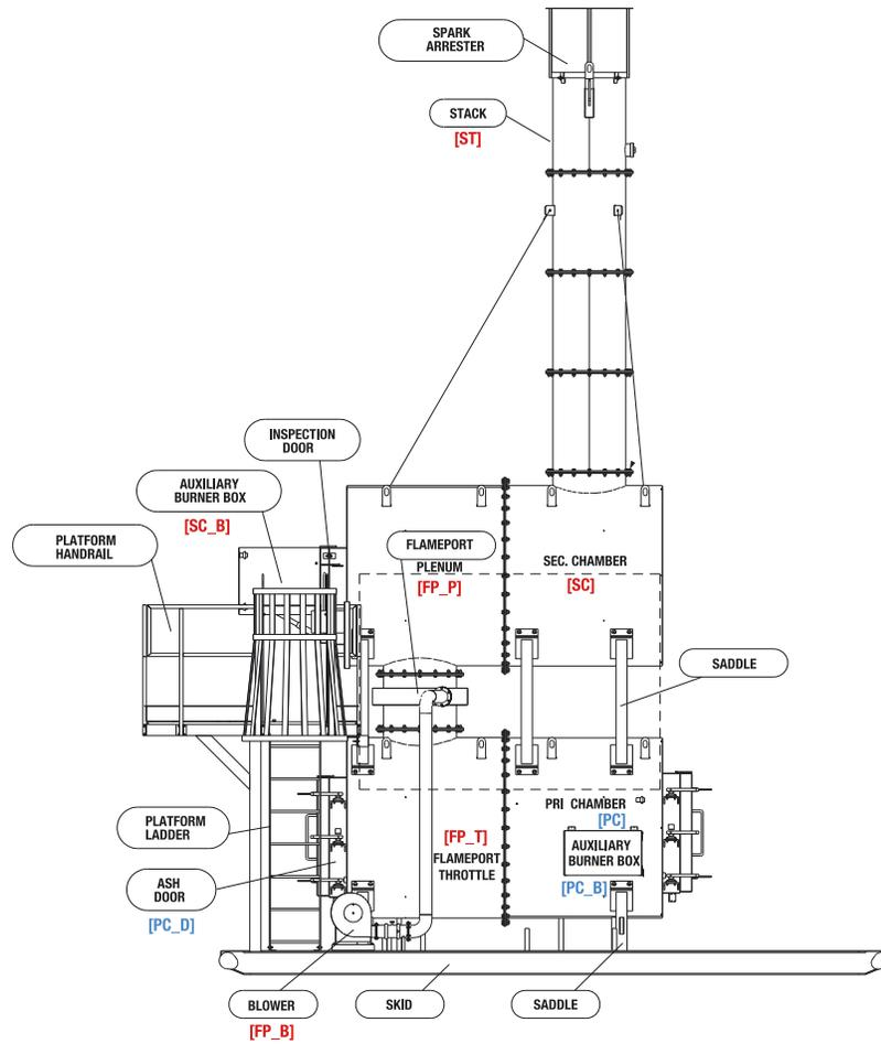
**FIGURE 6 COMPONENTS IN THE PRIMARY AND SECONDARY CHAMBER SECTIONS (1)**
