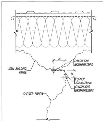
107.3 **CONNECTION BETWEEN SHELTER AND MAIN BUILDING** SCALE 1:5
