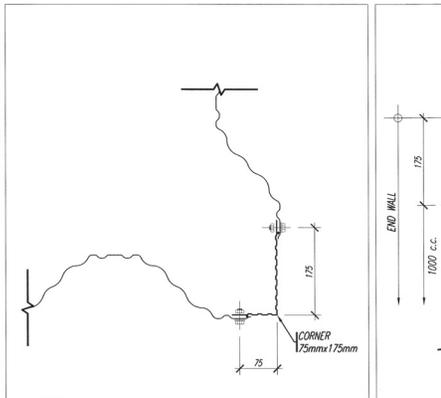
107.4 **TYPICAL CORNER DETAIL** SCALE 1:5
