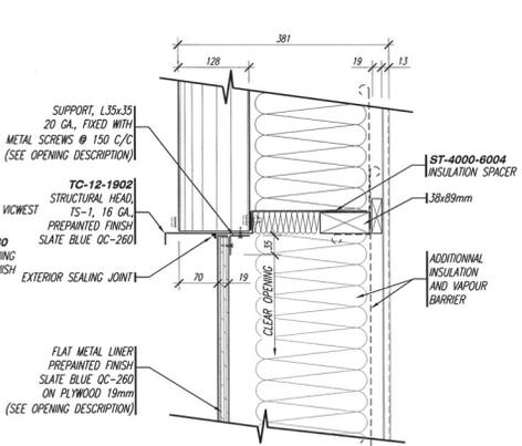
107.8 **HEADER ASSEMBLY FOR SPANDEL PANEL** SCALE 1:5
