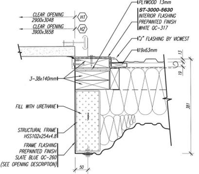
107.7 **VERTICAL ASSEMBLY FOR OVERHEAD DOOR** SCALE 1:5
