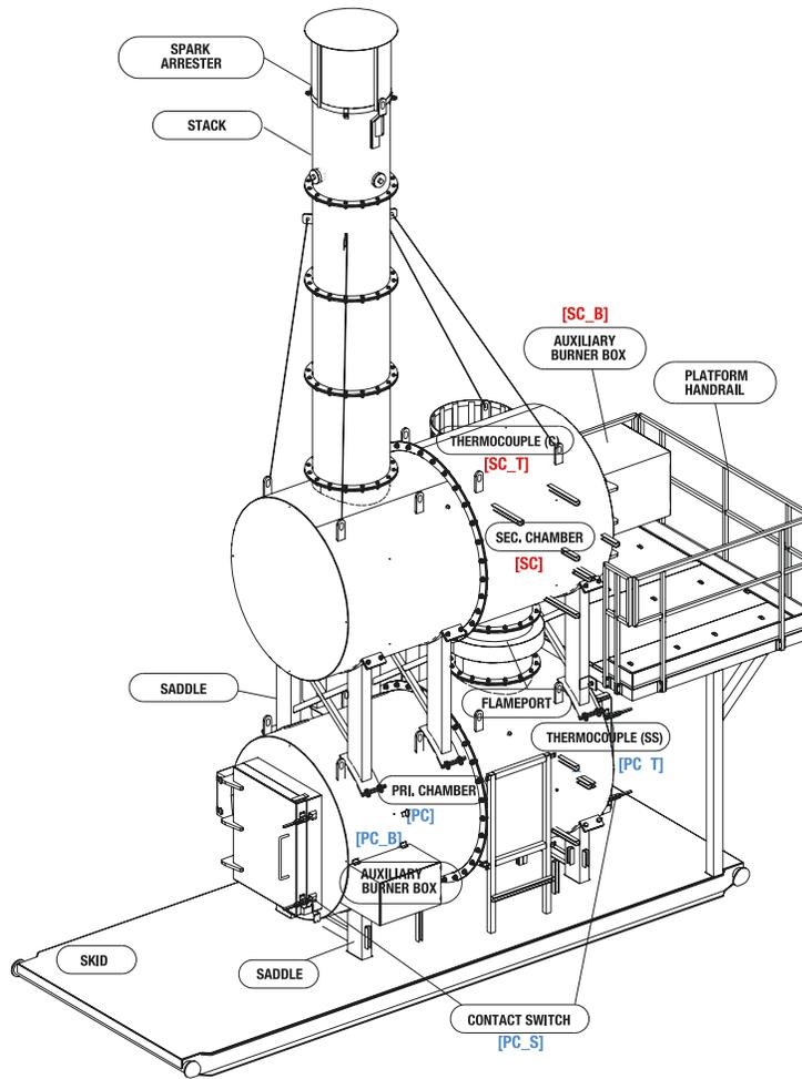
**FIGURE 7 COMPONENTS IN THE PRIMARY AND SECONDARY CHAMBER SECTIONS (2)**
