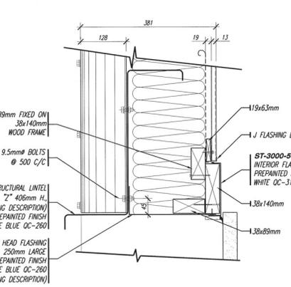
107.6 **HEADER ASSEMBLY FOR OVERHEAD DOOR** SCALE 1:5
