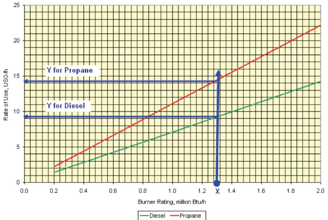
**FIGURE 13 CONSUMPTION RATES OF PROPANE AND DIESEL**
