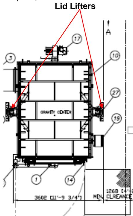
2. Once lifters are in place, shim and level, do not exceed 2.54 cm under the column. Anchor the columns to the floor.
