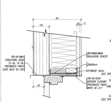
107.4 **HEAD ASSEMBLY FOR STEEL DOOR** SCALE 1:5
