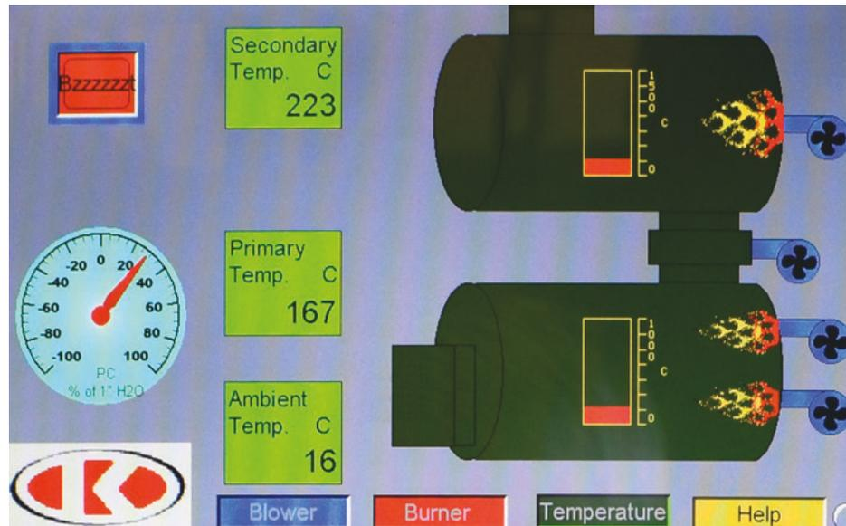
11. The temperature will keep increasing until it goes up to the set point and after that burners will continually function on/off to maintain the specified temperature set on the incinerator control system.
