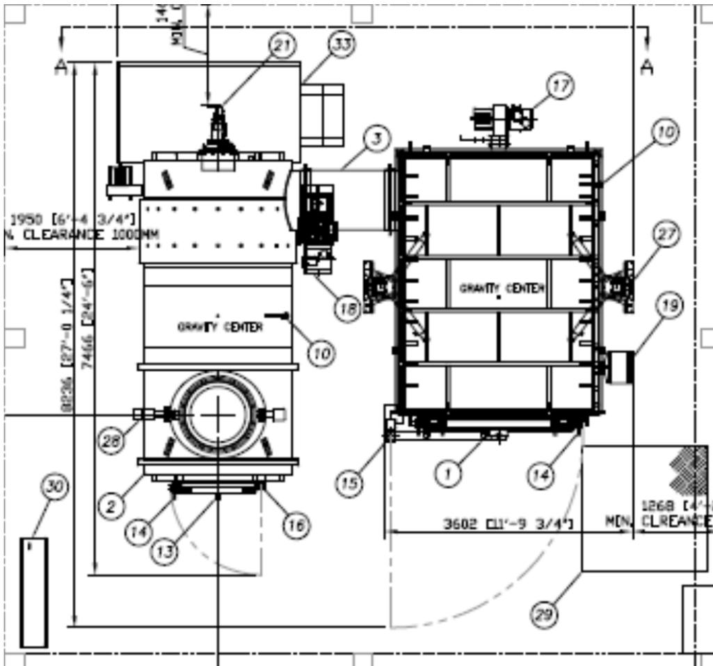
**NOTE** The diagram above shows the burners and blowers already attached to the Primary and Secondary Chambers. When positioning the Primary Chamber, Breech and Secondary Chamber, these items will not be attached.
