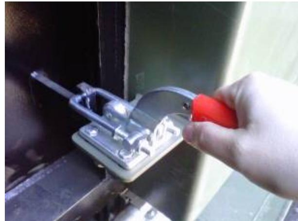
5. Ensure the Primary Chamber floor is cool (less than 90°C). Remove all the ash from the previous burn and store ash in ash bins.
