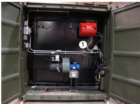
Primary Chamber Burner Flexible lines
