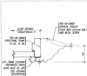
107.2 **VERTICAL ASSEMBLY FOR STEEL DOOR** SCALE 1:5
