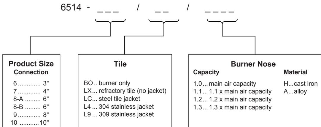
Example 1 6514-8-A/LC/1.2A Fireall gas burner complete with carbon steel jacketed tile and 1.2 capacity alloy nose
