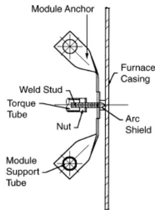
**Figure 1:** Side view of the Weld Loc Module
