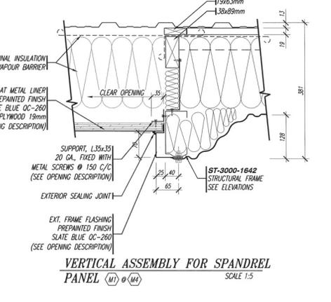
107.10 **VERTICAL ASSEMBLY FOR SPANDEL PANEL** SCALE 1:5
