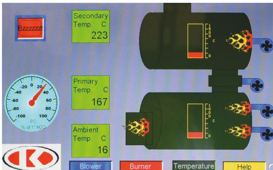
13. Approximately one hour after the rake, check the waste status again. If not burned, rake it and close the door. If waste seems burned and you do not need to burn another batch, then manually run the burn timer to zero. If you need to burn more batches, lower the set point on "Burn Timer" to 0 by pressing the "▲" down arrow. Give about 30-60 minutes for the Primary Chamber to cool down.
