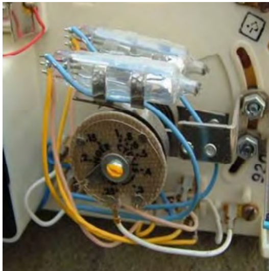
Figure 11 - Mercury-Containing Switches Source – California Department of Toxic Substances Control
