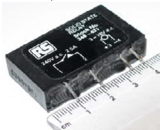
Figure 12 – Solid State Relay Switch
