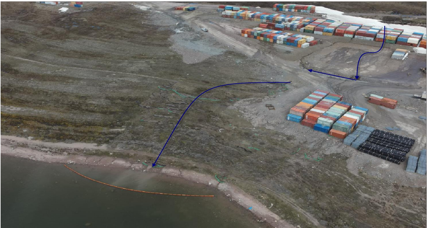
Figure 2. Aerial view of Baker Lake shore after Agnico Eagle's intervention and deployment of turbidity control measures showing the new flow path
