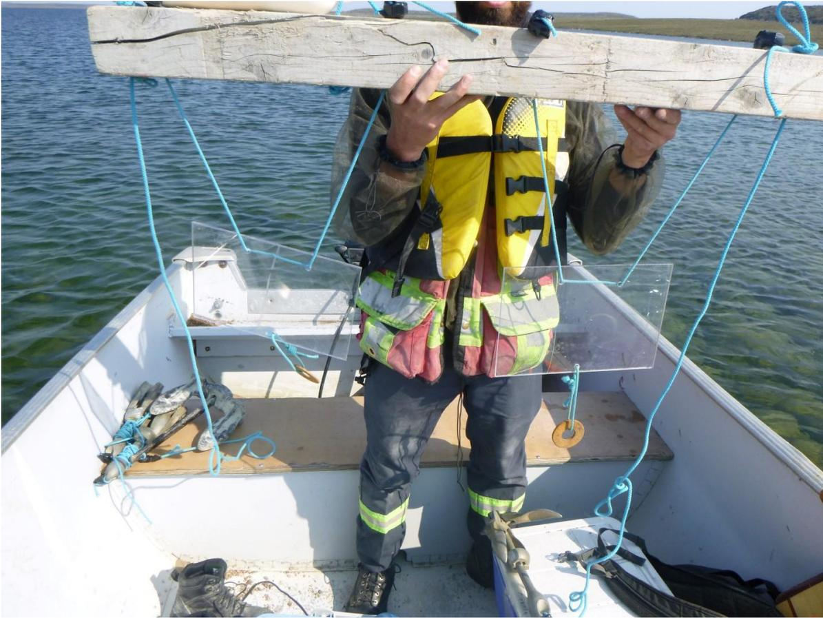
**Figure 3. Artificial substrate sampler for periphyton study in 2022.**
