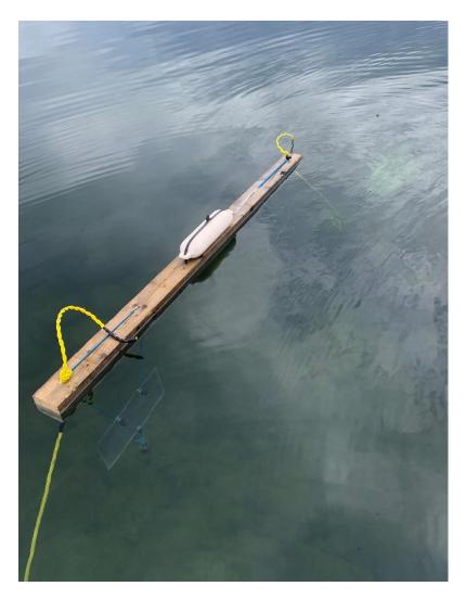
Figure 4. Artificial substrate periphyton sampler in-situ (2023).
