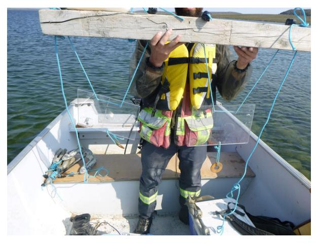
Figure 3. Artificial substrate sampler for periphyton study in 2022.
